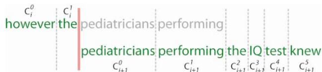
Figure 2. Merging two audio chunks with the optimal overlap point shown in solid red
