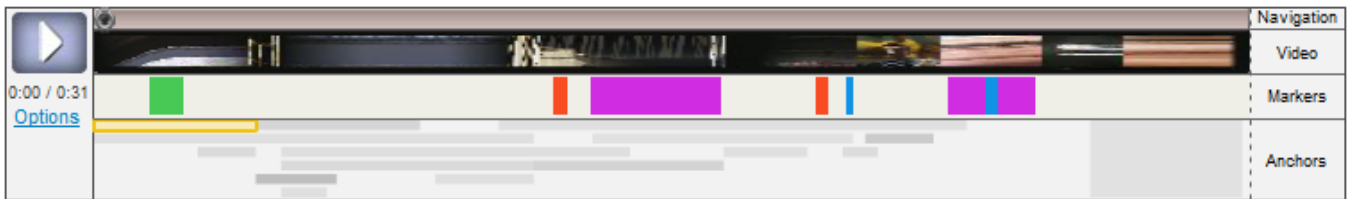
Figure 4. Stacked timeline view showing levels for navigation, stripe image, automatically extracted markers, and anchors.
